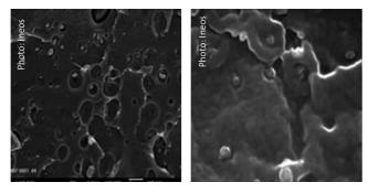
Electron microscope images of post-impact fracture surfaces of PVC foam. Left: Poor mechanical properties due to insufficient contact between nanoparticles and the foam material. Right: Good nanoparticleto-foam contact results in vastly improved impact strength.
